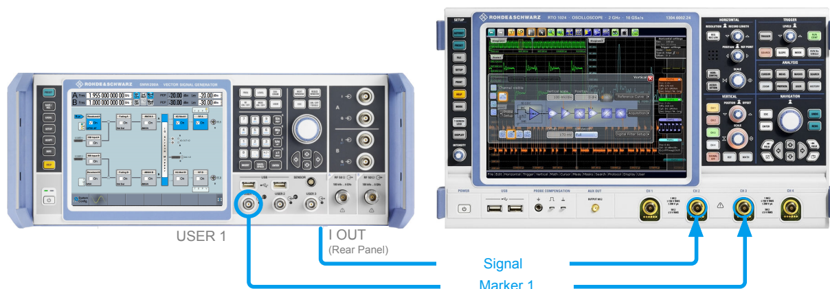
Figure 4-7: Simplified representation of a test setup for signal monitoring**
